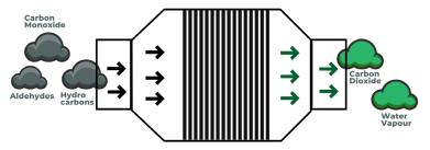
The effectiveness of the emission output is dictated by the <u>state of</u> the engine, the <u>temperature of the exhaust</u>, and <u>the composition of</u> the untreated exhaust gases. The **Flowtech Catalyst Combination Filter** necessitate a base temperature of around **180°C** (360°F) for the conversion process to initiate. Optimal catalytic performance is achieved at temperatures exceeding **250-300°C** (480-570°F).
